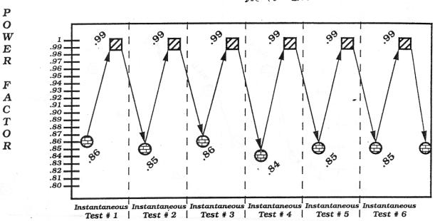
On this evaluation of the USES® CMES-3D 600 unit, off line the Power Factor reading off was .85.
